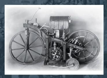
**Essential Components and Design:** The Reitwagen embodied the key elements that defined a motorcycle: a combustion engine, two wheels in-line, and a saddle for the rider. The engine, a single-cylinder, four-stroke design, was positioned beneath the rider's seat, and its power was transmitted to the rear wheel via a series of belts. The bike had no suspension, and steering was achieved by changing the wheel's direction manually.
